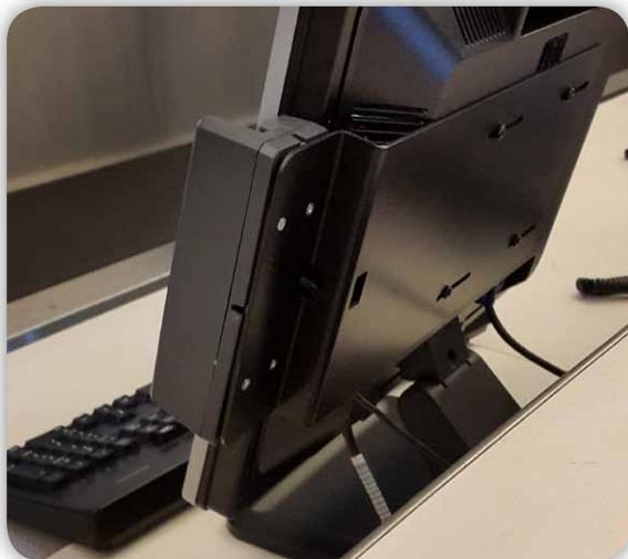
*Both readers can easily be attached to a range of devices. Above shown with option bracket for HP EliteDisplay 20"*
